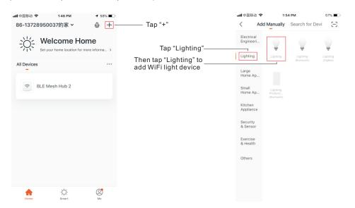
**Step 5:** Confirm that the WiFi LED controller is under connecting mode and configure it to the WiFi network which your smart phone or tablet connected to.
