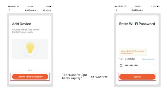
Step 6: Connecting starts, the WiFi LED controller will appear on the APP interface once added successfully.
